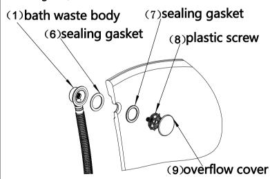
4. fill the bathtub with water and check for leaks.Place the bathtub in the prepared position, connect A side to the drainage pipe.Installation complete
