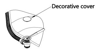
Click-clack functional failure is caused by the insert fault, insert should be replaced. Unscrew
